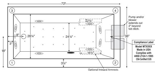
Numbered areas on tub deck represent possible locations to install cleaning systems, faucets and other fixtures. Pump extends out approximately 2" beyond tub deck.
